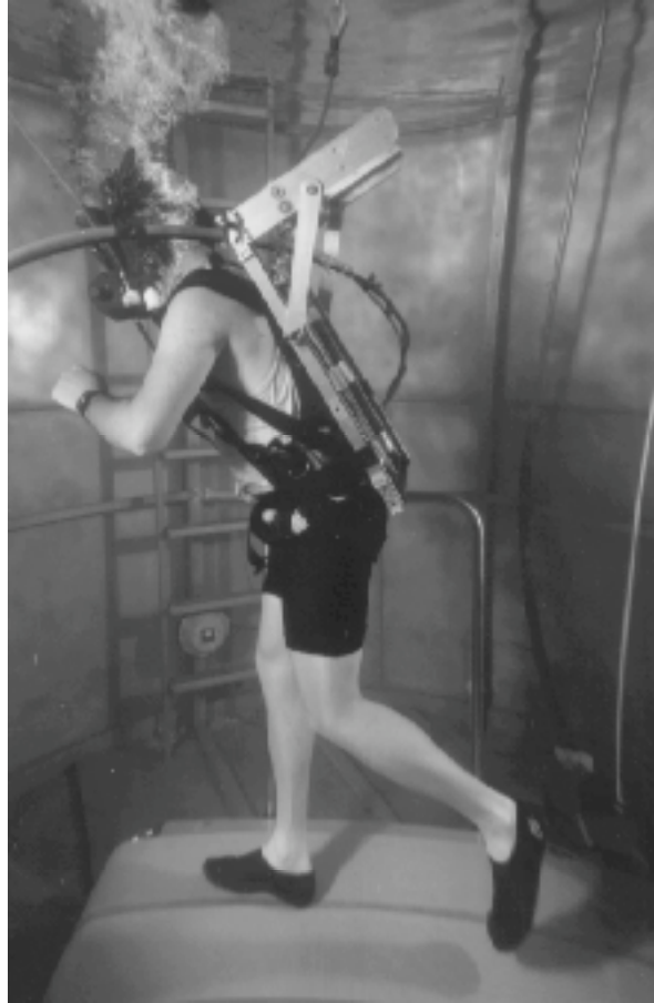
Figure 1. Subject wearing the Variable Position Load Backpack, with weight in the high back position.
